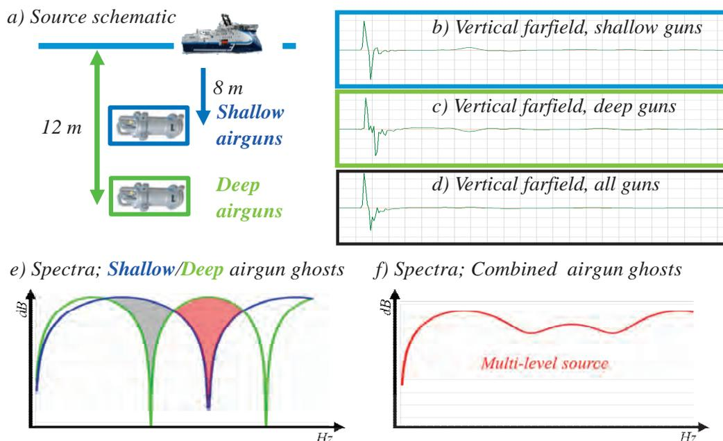
**Figure 1** Multi-level airgun source array layout, wavelets and spectra for shallow airguns at 8 m depth (blue), deep airguns at 12 m depth (green), and all airguns (red).
