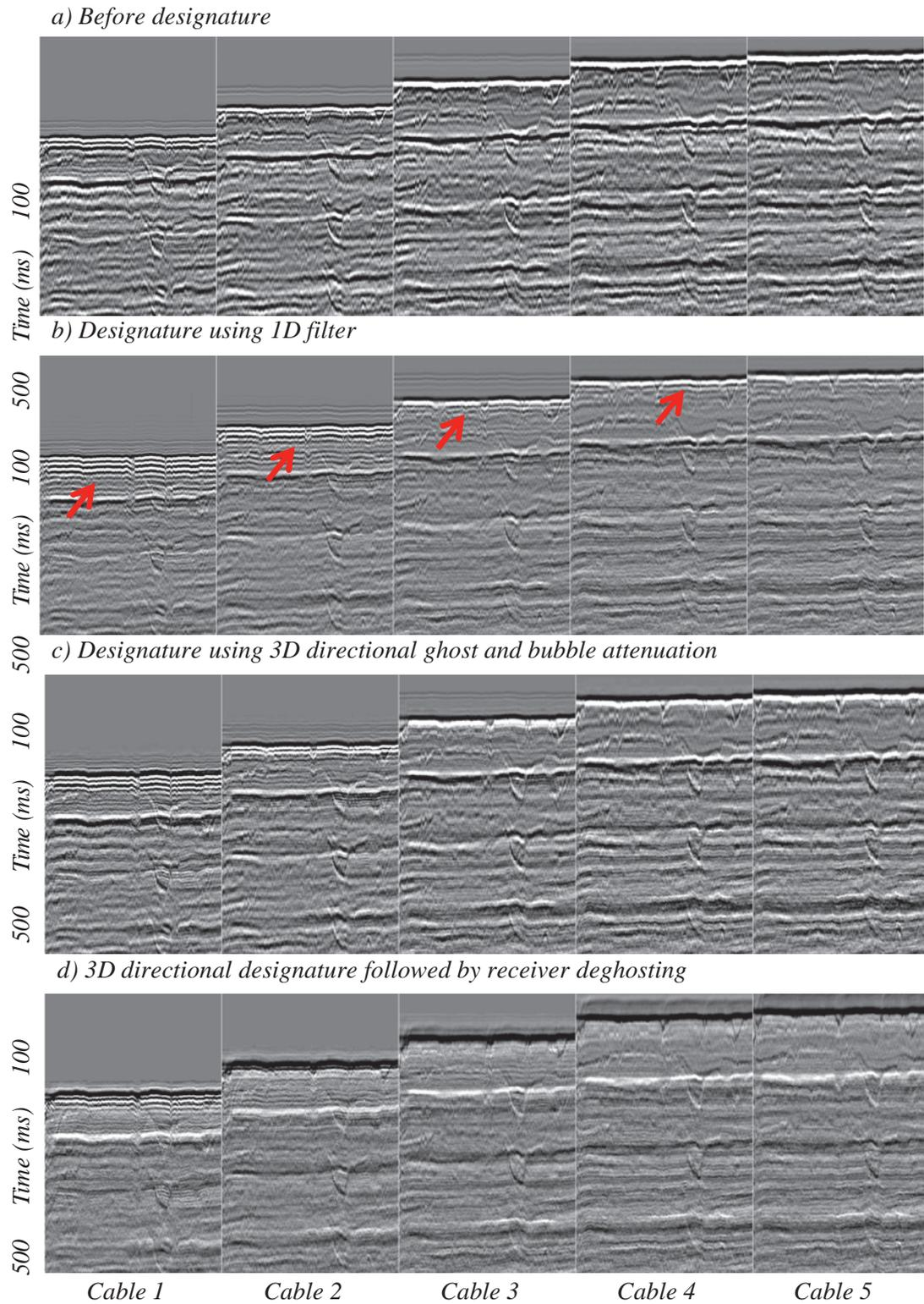
**Figure 2** Common channel displays for cable 1 (outer) to cable 5 (inner). Examples given for a) input, b) after 1D designature, c) after the proposed 3D directional designature, and d) 3D directional designature followed by receiver deghosting.
