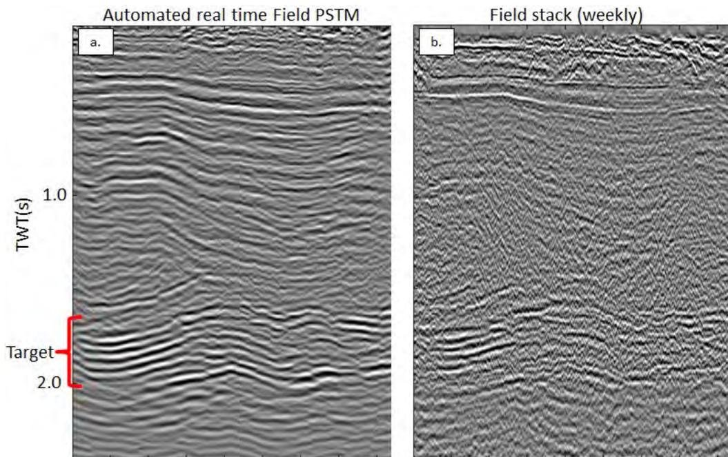
**Figure 4** Comparison of the seismic images obtained during the acquisition: automated real-time field PSTM (a) and field stack (b).
