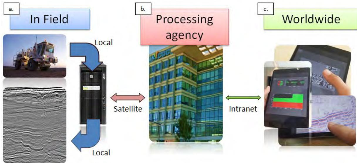
**Figure 2** Real-time automated field PSTM network.
