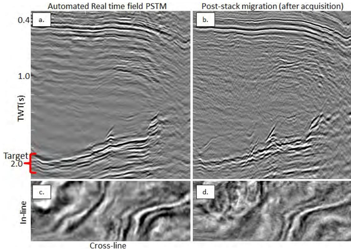
**Figure 5** Real-time field PSTM, (a) and (c), and the post-stack time migration, (b) and (d). Inline sections are displayed in (a) and (b). Time-slices at 2 seconds are shown in (c) and (d).
