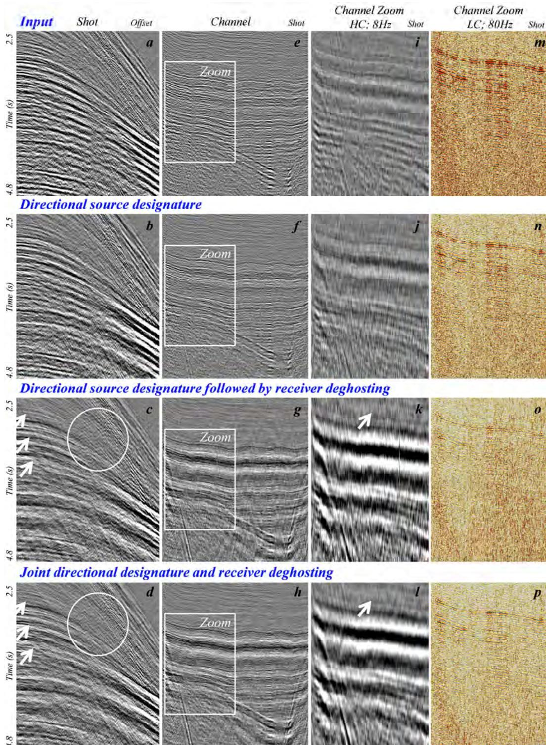
**Figure 2** Real data example comparing input, designature, sequential designature and receiver deghosting, and the proposed joint directional designature and receiver deghosting. Displays are given for shots (a,b,c,d), common channel (e,f,g,h), low frequency channel zoom (i,j,k,l), and high frequency channel zoom (m,n,o,p).
