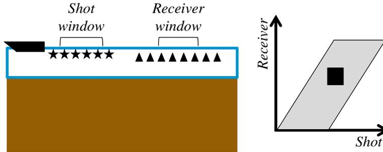
**Figure 1** Illustration of the shot-receiver domain, defined by a group of traces relating to shots firing within a spatially consistent shot window, recorded by receivers within a spatially consistent receiver window. This relates to a rectangular area in the shot-receiver stacking chart, right.
