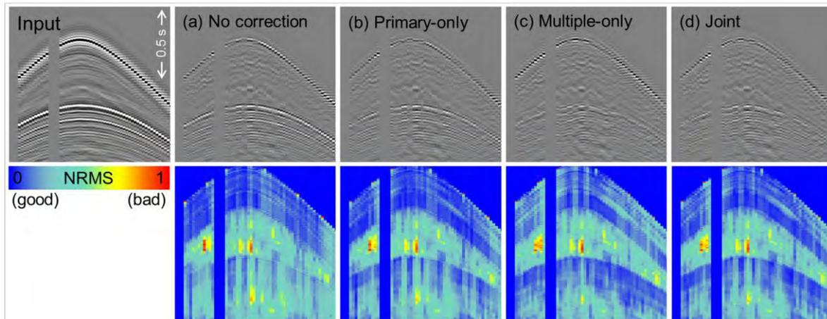
**Figure 3** Baseline OBN receiver gather (hydrophone) with 4D difference to monitor data (top) and NRMS plots (bottom) after different flavours of dynamic wavefield correction.
