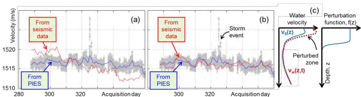
**Figure 2** (a) Measured (red) water velocity from seismic data using velocity parameterisation. (b) Using the depth-insensitive perturbation parameterisation depicted in (c). Blue lines are a running day-average of Pressure-Inverted Echo Sounder (PIES) measurements (grey).
