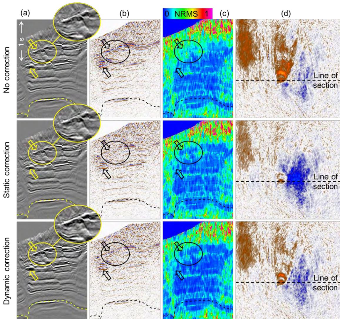
**Figure 4** Baseline images (a), 4D differences (b), NRMS (c) and amplitude from the 4D difference extracted on the dashed line (d). Inset detail highlights relative amplitudes on the baseline image.
