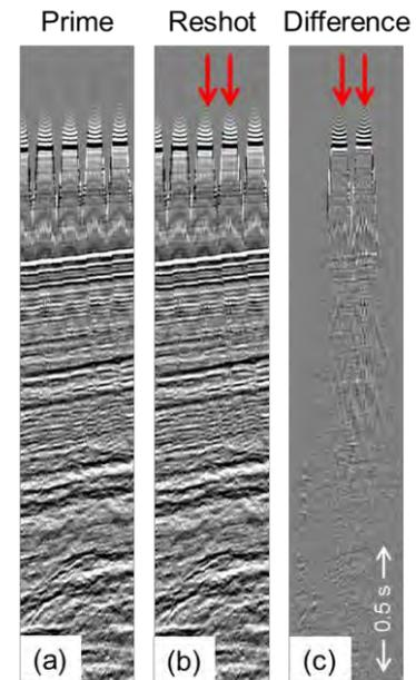
**Figure 1** (a) Baseline OBN stack. (b) Stack with two receivers (red arrows) replaced and reshot. (c) Difference between (a) and (b). Energy in the difference is dominantly caused by changes in water velocity.
