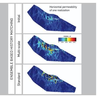
The porosity detail visible in the initial model (top) is preserved during the history match by EBMatch (middle) thanks to the multi-scale approach. A standard grid-blocked history match (bottom) results in loss of detail, which will impact flow simulation results
