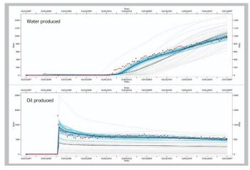
EBMatch updates multiple realizations of static reservoir grid properties (permeability, porosity, etc.) in order to improve the match to the observed production history data (red dots). The grey curves show flow simulation results of the realizations before, and the blue curves show the results after ensemble-based history matching of these multiple realizations of static properties. From Gentilhomme et al. 2015
