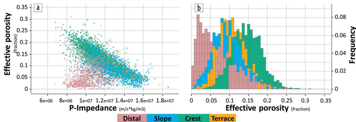
**Figure 3.** P-impedance versus effective porosity crossplot and effective porosity histogram from well logs, color coded by sedimentary environment facies for the various stratigraphic units analyzed in this case study. It is possible to see the trend for reservoir-prone facies in contrast with the profundal (distal) facies with lower porosities.
