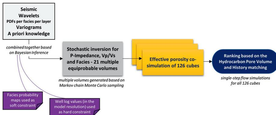
**Figure 5.** Simplified workflow that shows the main blocks of interaction and steps that enabled the closed-loop reservoir characterization and full static and dynamic integration in the streamlined production history matching. The image is based on proprietary expertise and interpretation from different works (Tehrani et al., 2016; Wang et al., 2016; Pendrel and Schouten, 2020).
