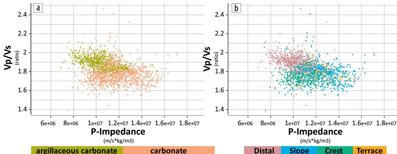
**Figure 2.** Facies analysis in the elastic domain showing crossplots of the P-impedance versus  $V_p/V_s$  ratio values from well logs, color coded by (a) facies types based on the free fluid porosity values and (b) sedimentary environment facies for the various stratigraphic units analyzed in this case study.
