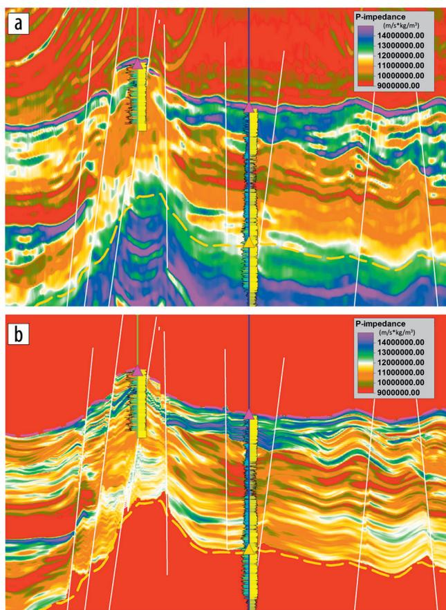
**Figure 10.** Comparison between (a) deterministic P-impedance result and (b) mean P-impedance from 21 realizations of the stochastic inversion. It is possible to see improvement in the resolution from the deterministic to the stochastic result. Also, the well logs (effective porosity and gamma ray at original sampling scale) enable the understanding and visual assessment of their variation in comparison with the main seismic-scale impedance contrasts.
