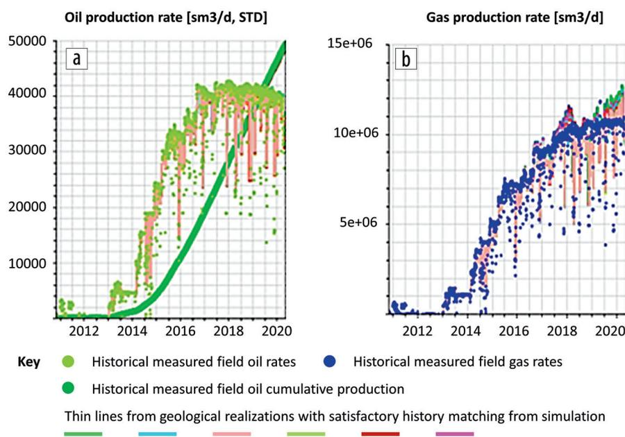
**Figure 12.** These two plots show the assisted history matching of oil and gas production. Both (a) oil and (b) gas production show the relationship between the history data and the geologic realizations, along with how this may be key to further improving the dynamic characterization of reservoirs.
