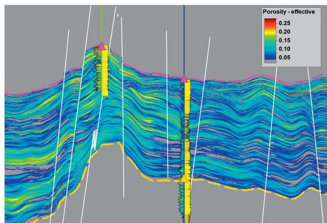
**Figure 11.** This section shows the most likely realization of effective porosity using HCPV ranking, which represents the input to the streamlined history matching. As in previous figures, the well logs (both effective porosity and gamma ray at original sampling scale) enable the understanding and visual assessment of their variation in comparison with the main seismic-scale effective porosity contrasts.
