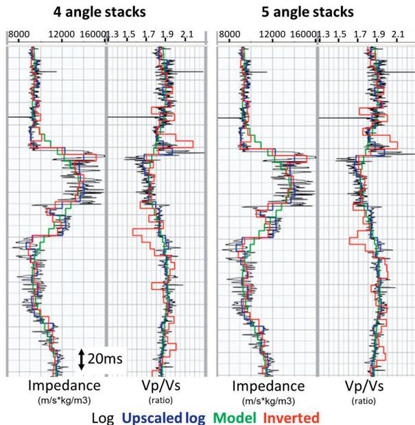
**Figure 4.** Elastic inversion test before and after angle stack optimization at one of the well locations that is representative of the whole study. It can be seen that the inverted impedance honors the well logs. It also shows how challenging it is to recover the  $V_p/V_s$  ratio for some parts.
