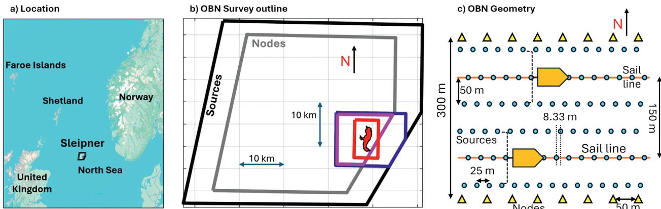
**Figure 2** Regional-scale OBN data acquired over the Sleipner field (a); the node and source footprint (b); and the OBN survey geometry with triple-source shooting over the ocean bottom nodes (c). The outline of the CO<sub>2</sub> plume is shown in red in (b).
