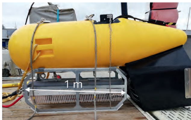
Figure 3 The sparker source used in the Conventional and Novel surveys.
